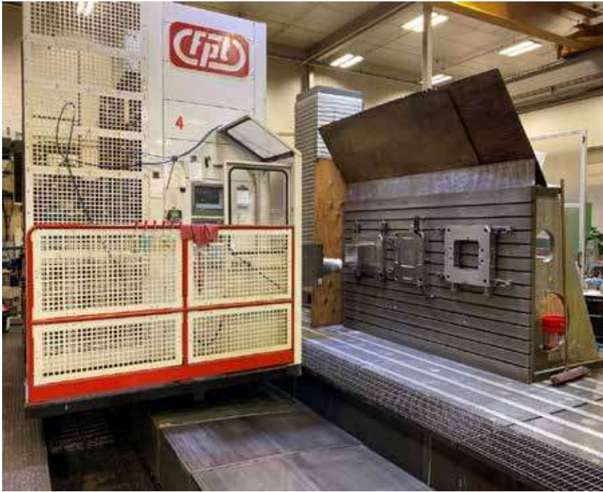
An example of the optimized manufacturing strategies employed by CDM, this FPT Pragma 3+2 horizontal machining center was set up and programmed to machine three individual mold plates.
